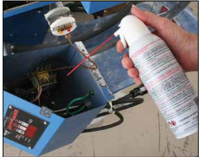
*Use canned air rather than a vacuum cleaner to remove dust from the inside of a kiln switch box. This is necessary only if you have the switch box open to change parts.*
