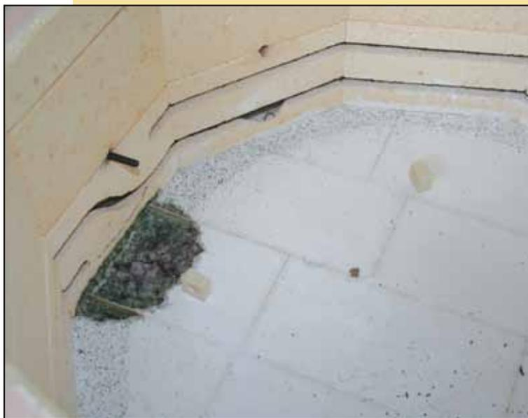
*The glass that has embedded into the firebrick floor can usually be repaired without replacing the floor. Note the missing sections of sidewall element groove and the element staple. This is minor damage that will not affect the firing results.*
