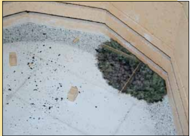
You may get a good deal on a damaged used kiln. Melted glass in the kiln bottom is often not difficult to repair.
