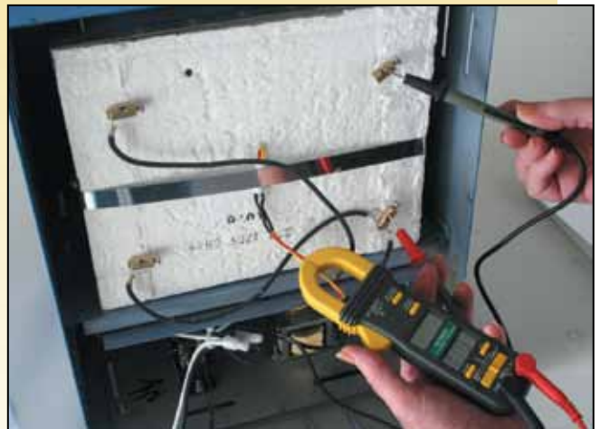
Before testing the elements with an ohmmeter, disconnect the kiln from the power.
