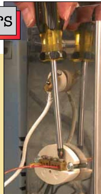
Before replacing a thermocouple or controller due to an erratic temperature display, make sure the thermocouple connections are tight.
