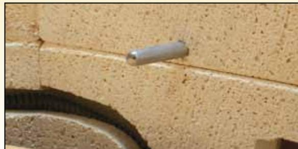
Before assuming that the controller is inaccurate, make sure any objects such as a shelf are not too close to the thermocouple. We recommend a distance of 1" between the shelf and the thermocouple.
