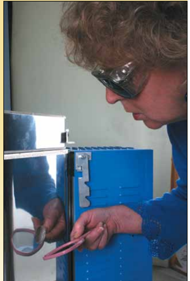
A mirror placed near a peephole sometimes aids in visually checking the kiln. Be sure to wear green #3 firing safety glasses when looking into the kiln.
