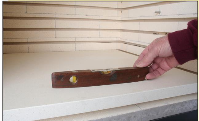
*If glass sags unevenly into a mold, place a small level across the shelf inside the kiln. Turn the level in several directions. To level the kiln, place sheet metal shims under the kiln stand. Make sure the kiln can't rock after you level it.*
