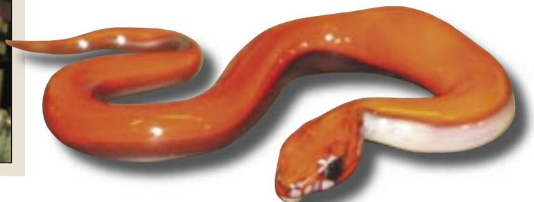
It's time for the final inspection. The paperweight is knocked off and annealed as follows: Hold at 980°F for 1 hour. Ramp down to 800°F over 8 hours, to 500°F over 6 hours, and to 70°F over 3 hours. This is for a double gob weight, or two 400 gram gobs. Jim anneals no more than two paperweights at a time, preferring to prevent shock by reducing the number of times the door is opened.
