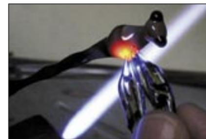
Once the wings are well centered and melted in, the final shaping of the wings is done. Use gradient heat to pull, shape, and tip the wings so that they are symmetrical.
