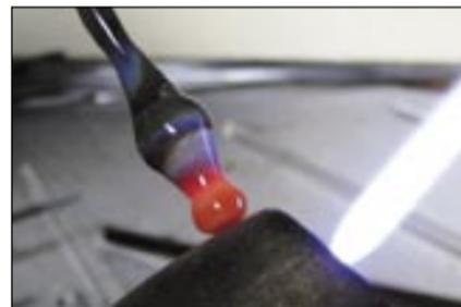
Flatten the top of the head, then round the bottom side of the head for the future loop area of the bail. I use the side of my torch for this.
