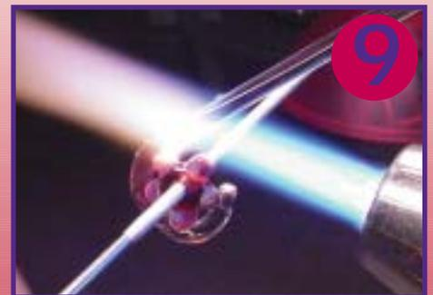
Continue bridging the dots by laying the glass over the tops without "pulling" the glass – just let the glass soften and bridge over the dots.
