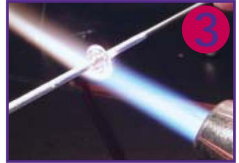
Melt outer surface of bead to make smooth. Bring the bead to the top part of the flame so that the flame licks the bottom part of the mandrel. It is important to keep the mandrel out of the direct flame for extended periods of time, or the mandrel will melt through, even with 320L rods. (Note: It is at this point that you can round off your bead and finish it as a spacer.)
