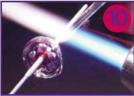
Continue applying glass over the first layer for a total of two layers.
