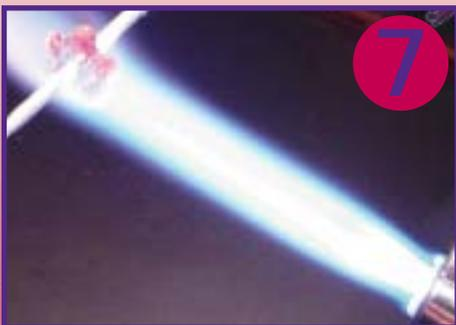
Increase the propane to the torch so that you have a reduction flame. Spin bead in this flame until a dark, grape/purple color appears on the dots. (Note: Stopping at this point will give you a second style of bead.)
