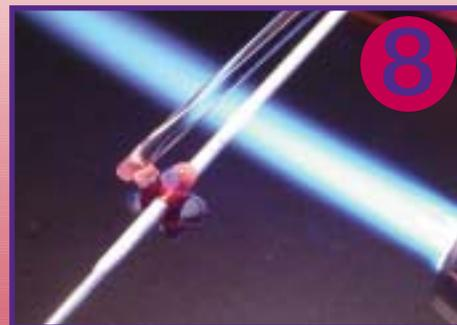
Bring torch back to a neutral flame. Using the 5 mm Symax rod, heat the end and place on the full face/top of a dot.
