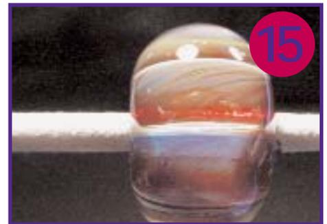
Put back into the far reaches of the flame to strike again until the trapped haze from the reduction of the Northstar Double-Amber Purple (NS-26) dots starts changing into a myriad of colors.
