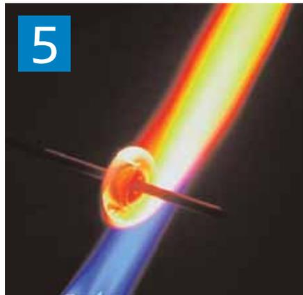
5 Then, place bead into the flame to melt until smooth. Continue turning the mandrel to heat the entire bead evenly. Allow the bead to cool until the entire orange glow is gone.
