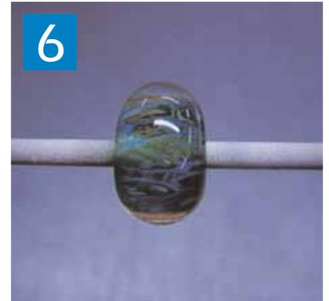
6 Then flash the bead in the outer flame until the color strikes. You will see the bead getting darker in color as it begins to strike. Place the mandrel with bead on it into the kiln to be annealed.
