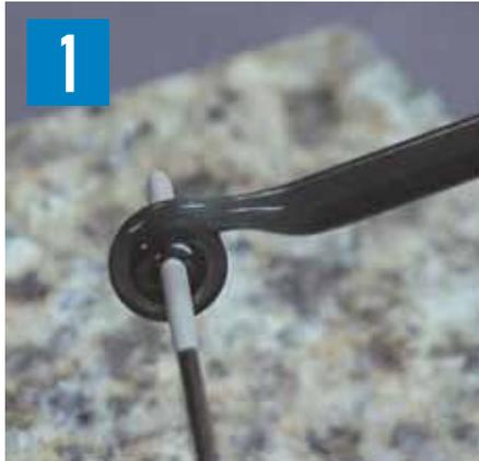
1 While holding the mandrel just under the flame, heat the teal sparkle until it is molten. Wrap the teal sparkle twice around the mandrel. Continue turning the mandrel to heat the entire bead evenly.
