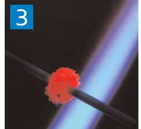
3 Return the bead to the flame and rotate the mandrel to heat the bead and melt the frit evenly into the surface of the glass.
