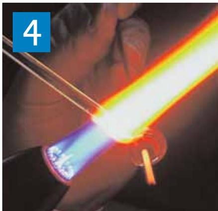
4 Next, encase the bead in three layers of clear, being careful not to trap any air bubbles.
