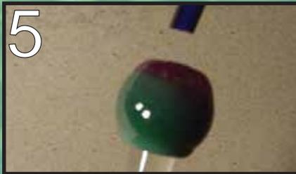
5 While the surface is still hot, and you are able to move the cane around, do so in a back and forth motion once or twice, but stop before the cane becomes too stiff. Pause for 3 or 4 seconds, then snap the cane off to one side with a sharp motion.
