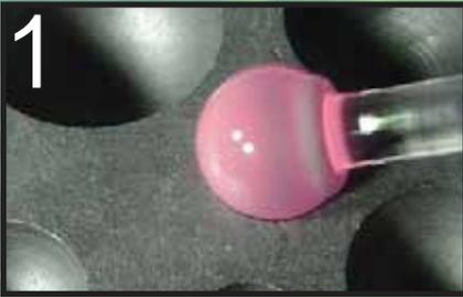
1 After applying a base color, use a marble mold to shape. By shaping the marble before applying the murrini, the images won't be distorted by the manipulation.
