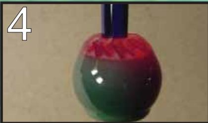
4 Heat up a small area on the marble until white hot, then stick the murrini cane into the surface of the marble about 2 or 3mm. This one is in the middle of the ribbon cane.
