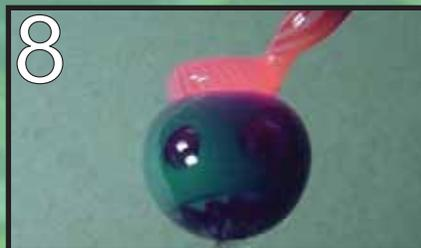
8 Apply a punty, and separate the clear rod, making sure that no clear is left behind. Accent with more filigree (on this side I chose surface striped cane) then melt in. Apply another murrini, cover with the dab of clear and melt.
