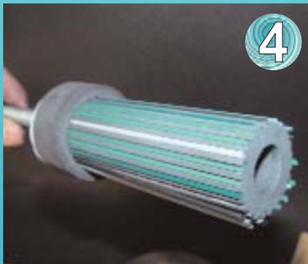
Blind holes at the end near the handle hold the sticks in place.
