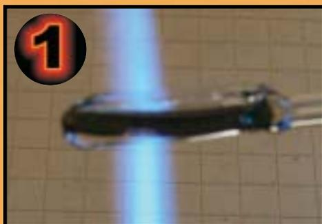
Begin with a section of color about 1" long attached to a clear handle. Draw 2 or 3 lines down the color with clear. **Tips:** By warming the color section before adding the clear will give the piece different characteristics resulting in more contrasting colors and defined patterns in the final mix.
