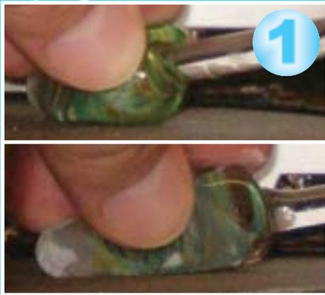
I usually start off with the 100 mesh disk to facet the largest areas first and to obtain the general shape of the piece. The smaller facets (typically known as points) are done on the finest diamond wheel because the surface of the 100-mesh wheel is too abrasive and will chip the edges off of the finer points.
