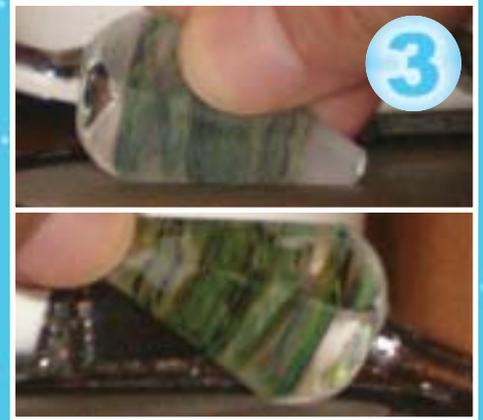
After I have completed the major shaping I move to the 260 mesh diamond wheel going over previous facets to remove ridges left behind by previous wheel. Moving the piece around the wheel and using a lighter touch will avoid deep surface scratches and pattern from developing. This will cut down on the time it takes during the final polishing process.
