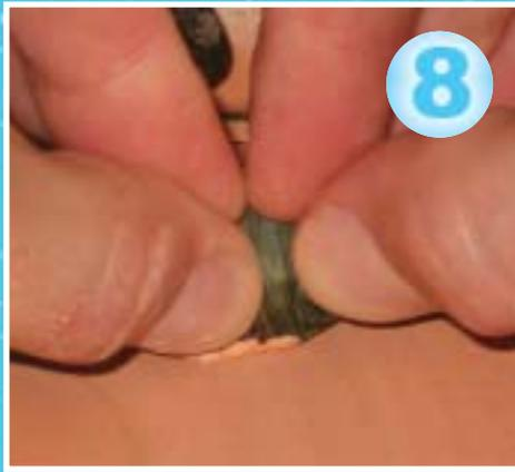
The final polishing is done using a felt wheel imbedded with Cerium Oxide. I run the wheel at 1-2 drops every 2 seconds with a fresh coat of Cerium Oxide applied.
