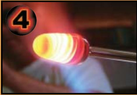
Now start heating the left hand side of the section and as the glass becomes fluid begin pulling and stretching this area gradually working your way down to the area you wish to separate. The shape of our section should now resemble a cone. There are many possibilities for different shapes at this point. Use your imagination and experiment, then go with what you like. Personality brings out a piece and others will appreciate an honest effort.
