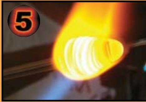
The next step is to begin heating the piece concentrating the flame on the area with the greatest mass. This will allow you ample time while marvering. Be careful. Too little heat will leave you with a sloppy, labored and inconsistent marvering job while too much heat will tend to distort the shape and possibly make your piece flop around minimizing the control you will have while shaping.
