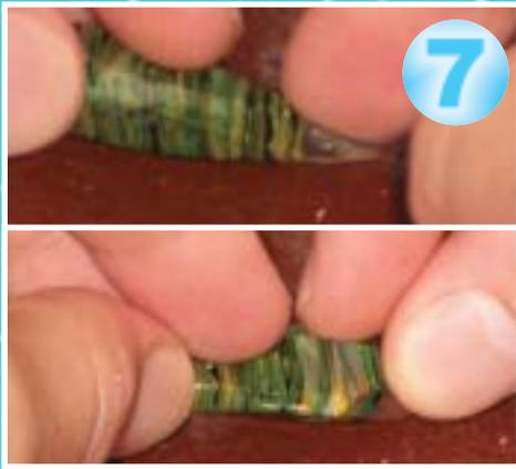
The next step is to begin polishing the piece bringing out the potential brilliance behind the rough finish left by the diamond wheels. Using the 325 mesh smoothing disk start by polishing the largest surfaces first gradually buffing out the area resulting in a very, smooth, matte finish.
