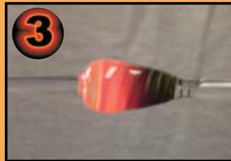
Next, gather up the right side of the mixed color section. This will end up being the top of the arrowhead. Afterwards when the piece is finished, a loop can easily be attached to turn your work into an extremely attractive centerpiece of a necklace arrangement.
