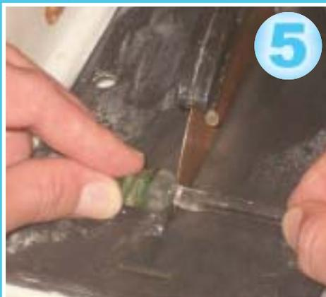
Once you have finished getting the major faceting done the next step is to remove your handle. For this step I use a wet cutoff saw. Remember to wear eye protection because glass can go flying off during this step.
