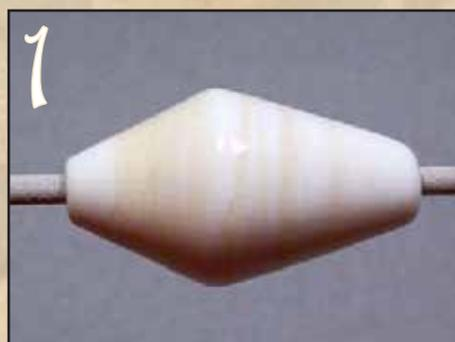
Using your ivory rod, wind enough glass onto your mandrel for the size bead you want. Marver it into an off centered bicone shape with a shorter side, which will be the top of the shell, and a longer side which will be the bottom of the shell. If you decide to add decorations such as melted in dots or stripes, do it at this point and then heat and reshape your bead back to your off centered bicone.
