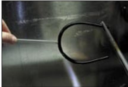
Puncture with a cold seal and bend gently into a horseshoe.
