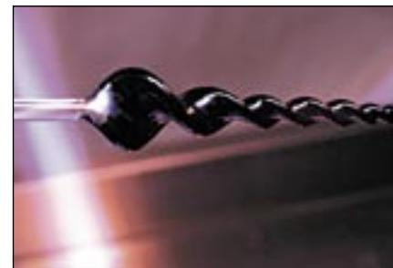
Remove the punty from the top of the twist. Garage in the kiln.
