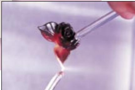
Adjust the leaves as desired. Reheat and garage in the kiln.
