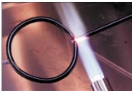
Bend into a complete circle, fuse onto the remaining Jet rod, and garage in the kiln.
