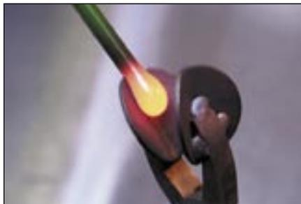
Heat the green rod and smash the drop with the angled, veined masher.
