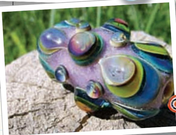
**4/18/08** Tried to reduce. Had to do a little research on how to reduce with this setup. Oh, lower the oxygen, bushy flame; I see. Wow! Look at that reaction! Some silver glass just needs a kiss of the reduction flame, some needs more. I bought a sample pack of different types of silver glass to see which ones I like. Glad I did this, because there are two I really like a lot!
