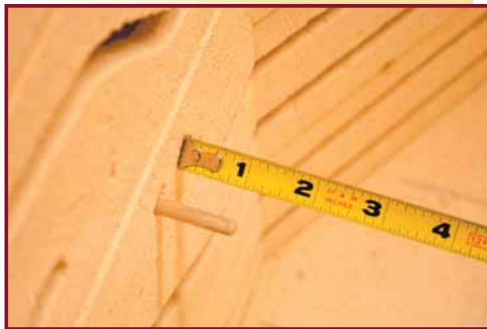
The thermocouple measures the temperature inside the kiln.
