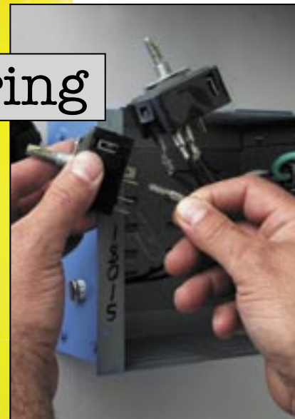
Firefly switch replacement C1. Make sure the connections are tight when you replace electrical components.
