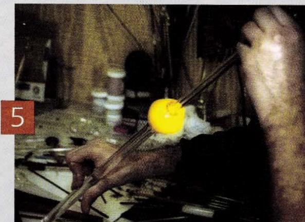
5. The rod is now about 32 mm thick and ready to be heated and blown out. This is the fun part. I gather the mass into a round ball at the end of my punty rod. Because the color is encased in a nice transparent, I do not need to consider atmosphere in my flame. All I need to do is get it HOT, really hot.
