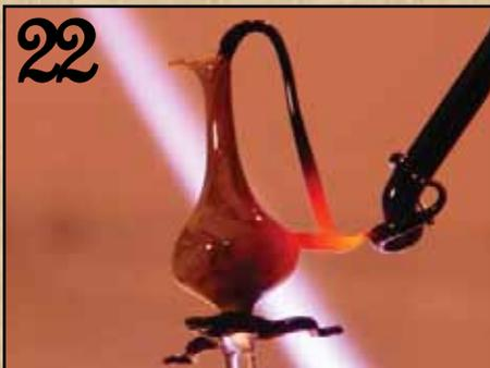
22 Using a pinpoint flame, weld the bit from step 19 and the handle. Tug and pull material to reach the desired flow.
