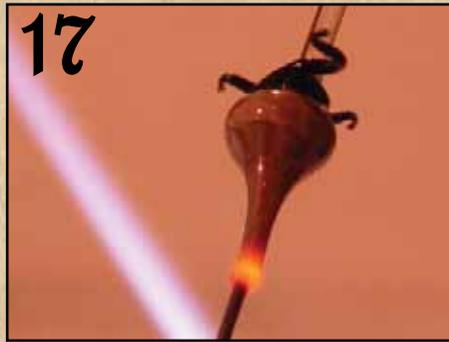
17 Use a tungsten pick to open the "mouth" of the vessel. Flare it slightly.
