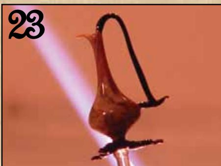
23 Flame anneal the vessel. Then detach from punty and heal the punty mark. Get 'er in the oven, pronto!
