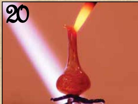
20 Using 7mm color rod, heat 1" of rod and tack lightly to the neck, opposite the spout and directly above the bit in step 19.
