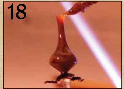
18 Heat and pull a portion of the flare to serve as the spout of the vessel.
