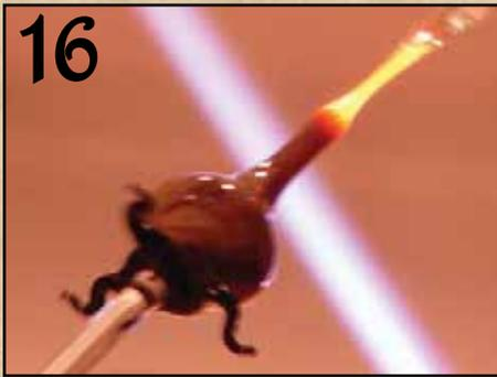
16 Using a pinpoint flame, heat then stretch and separate the neck. Use clippers to open the vessel.
