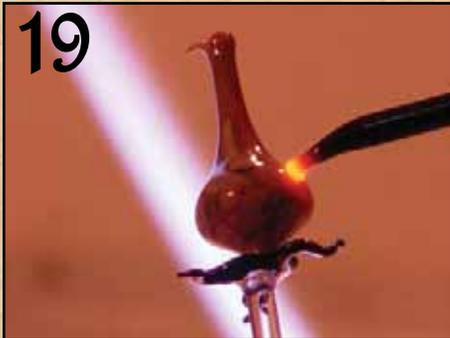
19 Attach a small bit opposite the spout on the backside of the vessel. This is an attachment for the handle.
