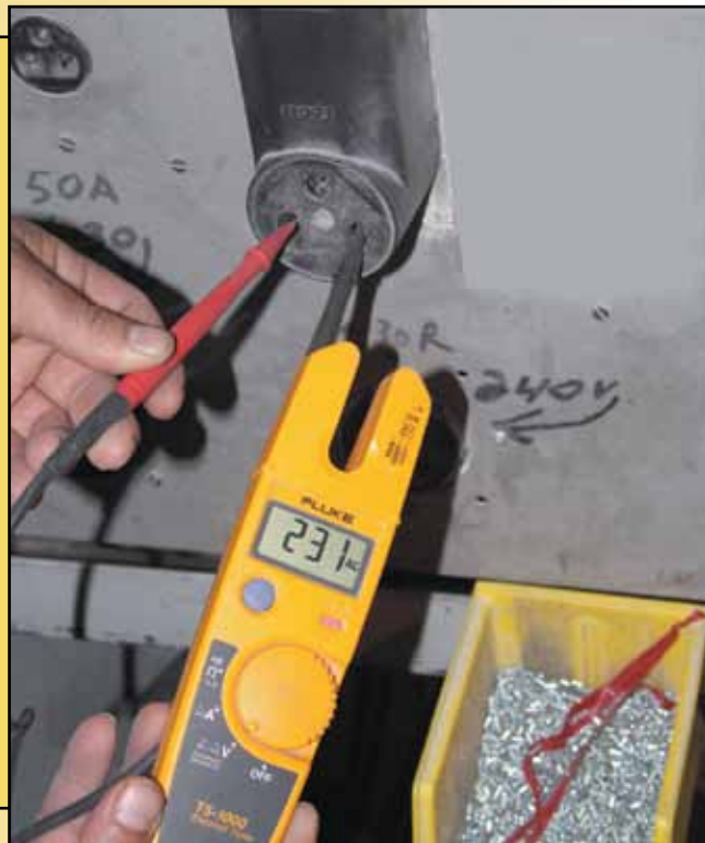
Use a voltmeter to test wall outlets and an ohmmeter to test elements. The multimeter shown here has three modes--voltmeter, ohmmeter, and ammeter.
