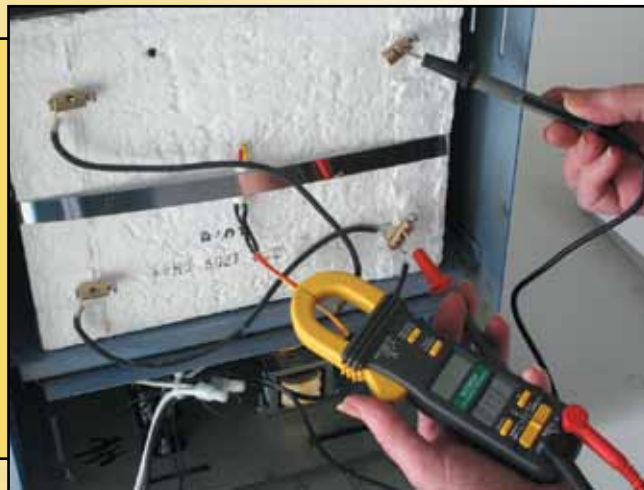
Shown here is a 120-volt SC-2 kiln that has two elements wired in parallel. Note that the two wires have been disconnected from the upper right element connector before testing with an ohmmeter. This was necessary to prevent the ohmmeter from giving a false reading.
