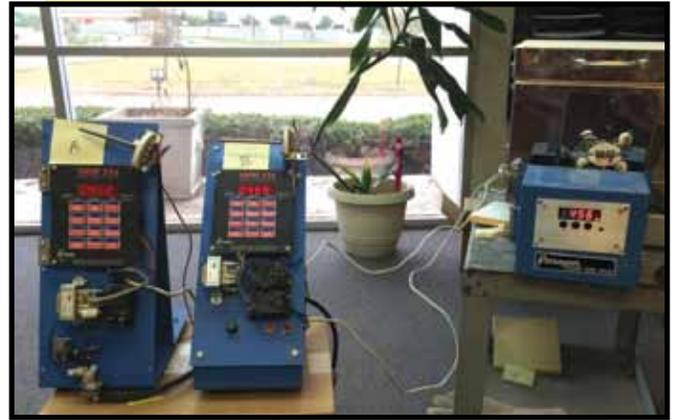
*In this photo, three controllers show temperatures of 452°F, 469°F, and 456°F. The three thermocouples in the test kiln each give a slightly different reading because of the differences in positioning in the kiln and the thickness of the thermocouple tips.*
